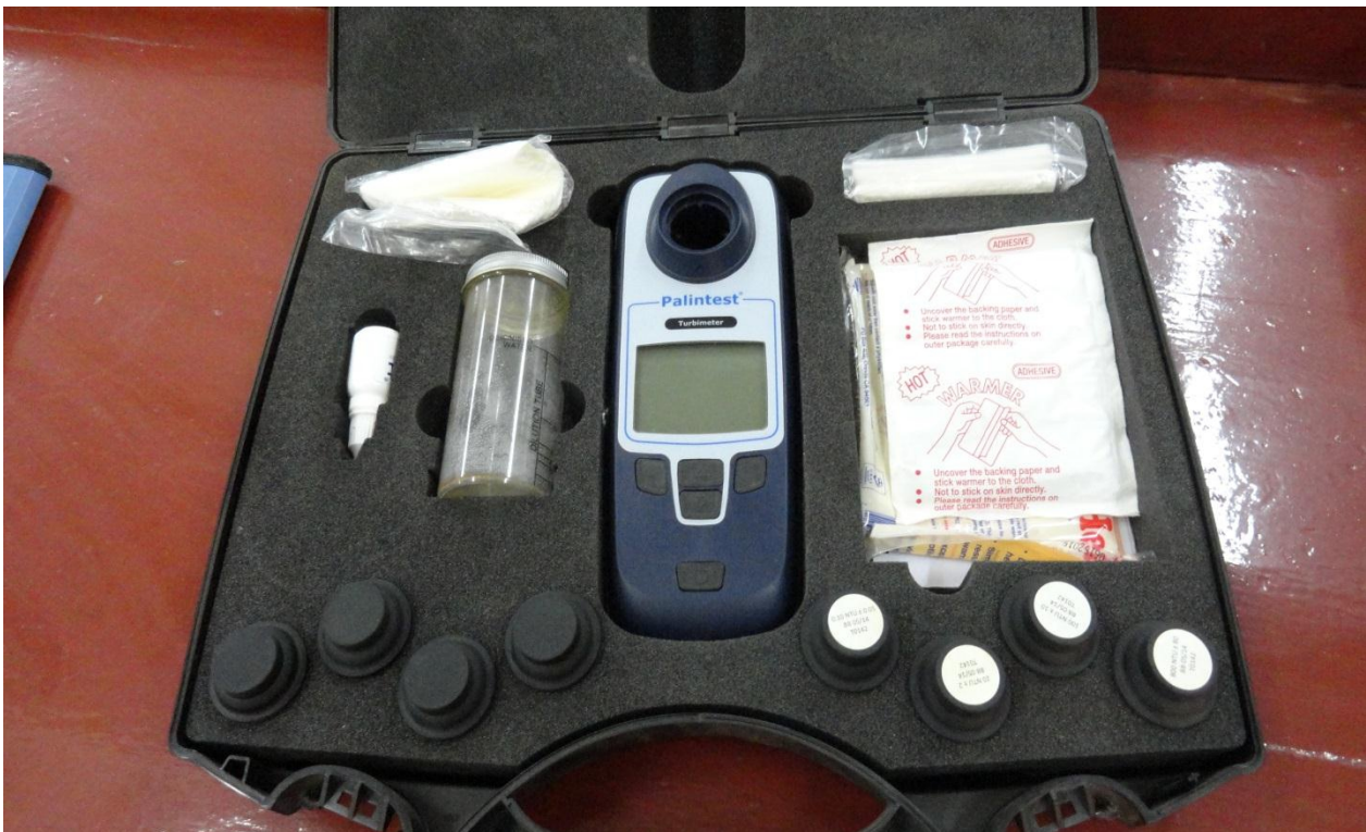
Plate (3) Turbimeter used in measurement of water turbidity.
