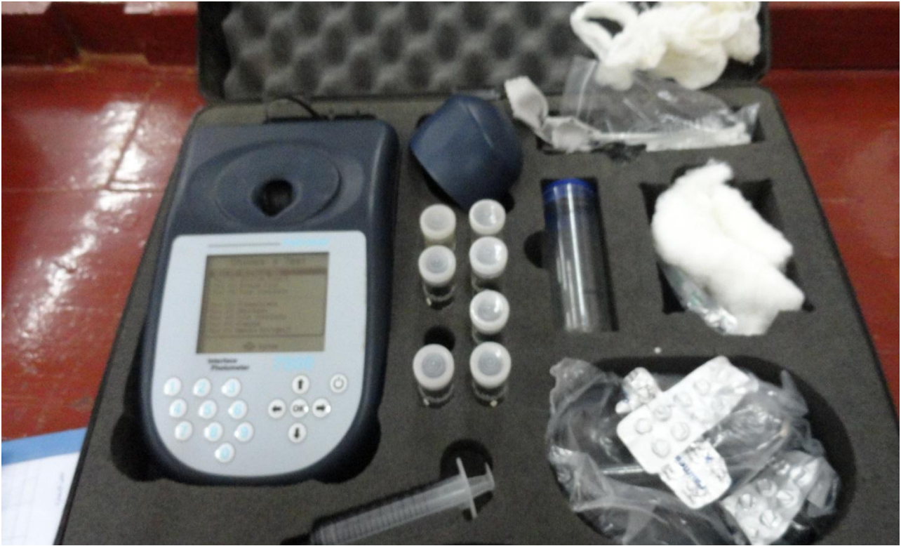
Plate (1) Photo meter that used in chemical tests.
