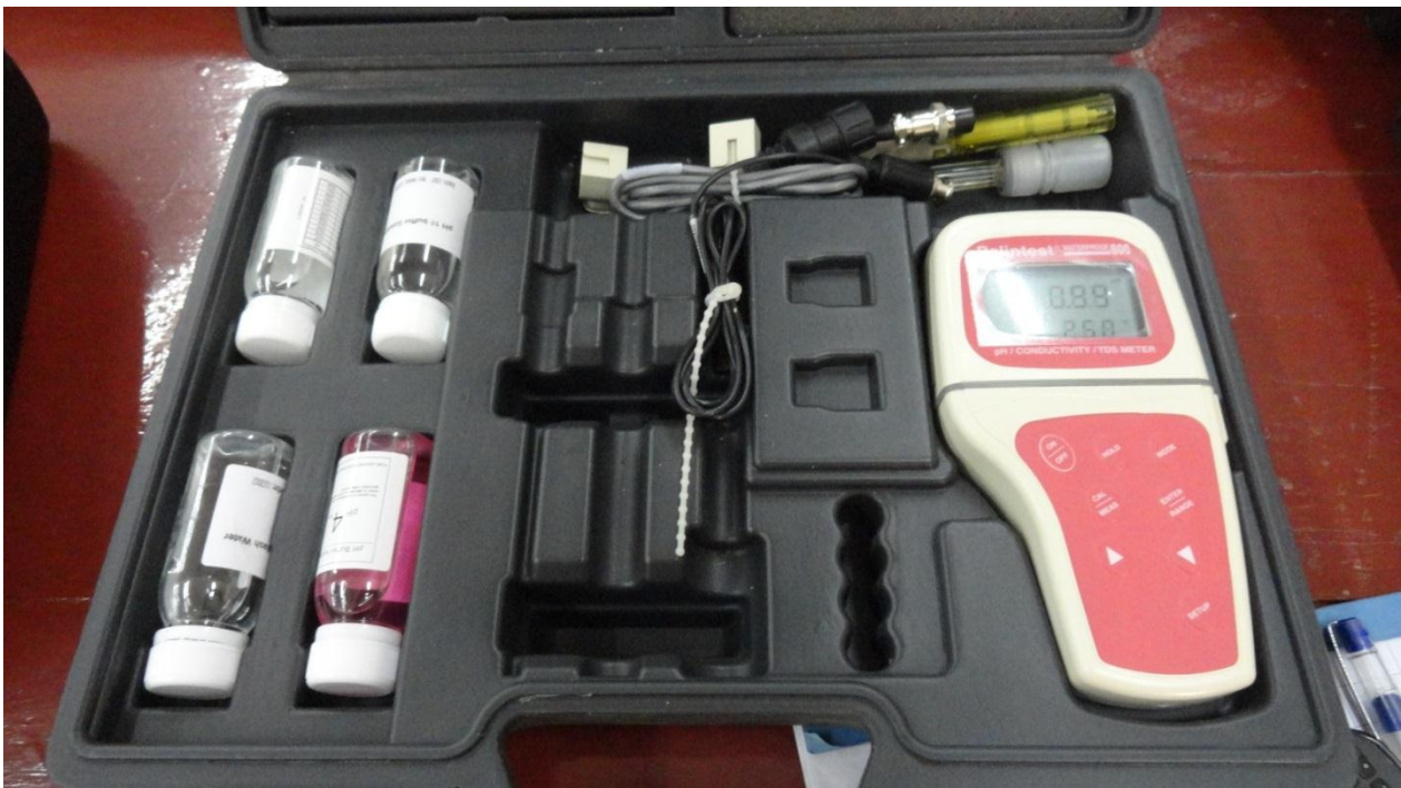
Plate (2) conduct/ TDS meter used in measurement of conductivity/ TDS of water.
