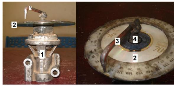
Fig (3): EGR valve. 1- EGR valve. 2 – 360deg. Protractor. 3 – Pointer. 4- Rotating bolt.
