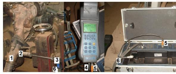
Fig (2): Flue gas analyzer. 1- Exhaust pipe. 2- Metal hole. 3- Steel tube and handle. 4- RCU power supply. 5- Communication cable. 6- Gas suction hose. 7- MCU power supply.
