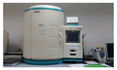
Figure 4. BDPhoenix 100,automated system for the identification and susceptibility testing of clinically relevant bacteria from Bicton Dickinson company, US.
