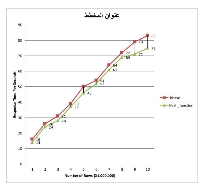
Figure 4.9 response time from HBase and hash function
