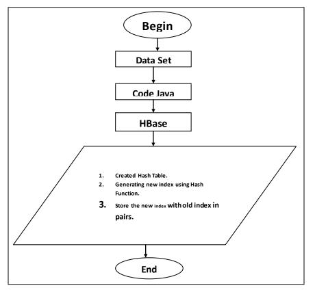
Figure 4.4 Flow chart Store Data in HBase using Hashing
